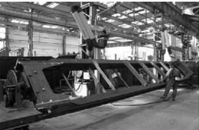
Frames, masts, booms and cabins for material handling equipment
