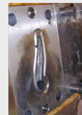
Brass handles are pressed in a Toolox® 44 die in one stroke at 730-750°C.
