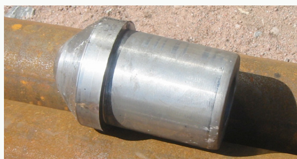
Figure 12. Example of an adapter between the striker of the hydraulic ram and the pile during impact.
