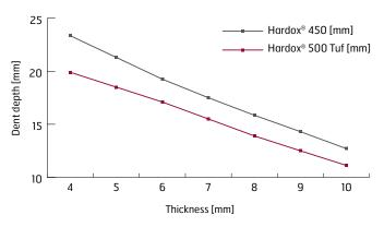
Results from impact drop tests of Hardox<sup>®</sup> 500 Tuf and Hardox<sup>®</sup> 450.
