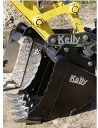
Quick couplers from Kelly Attachments rely on Hardox® round bars for toughness and long service life.
