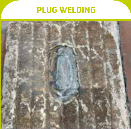
Use 560 MPa (80 ksi) low carbon joining wire to fill the base of the hole.
