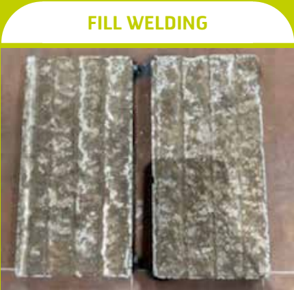
Before welding two pieces of 10 mm on 10 mm (3/8" on 3/8") Duroxite® 200.
