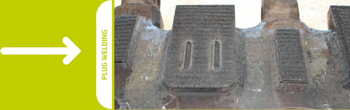
Plug filling of the oval hole when attaching a piece of Duroxite® plate to an excavator bucket.
