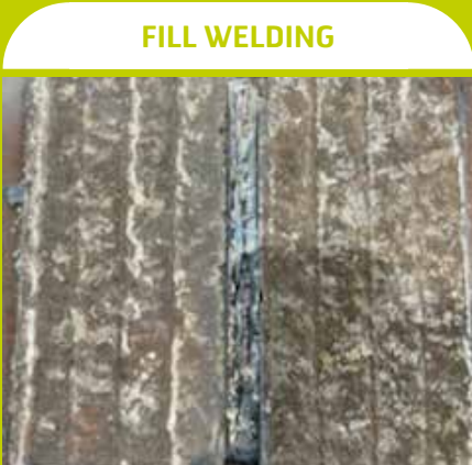
Use 560 MPa (80 ksi) low carbon wire to join mild steel substrate of Duroxite® 200.
