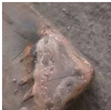
Thicker overlay is welded away from the corner, thinner overlay at the edge.
