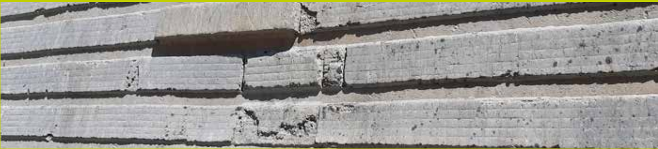
Spalling has occurred on edges of the liner plates because the gap between the liners was not properly filled with hardfacing wire.
