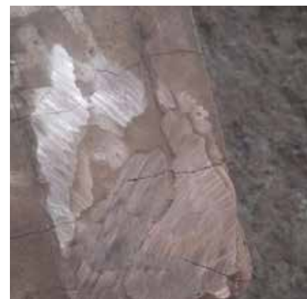
The repaired surface should be ground to become smooth and round.
