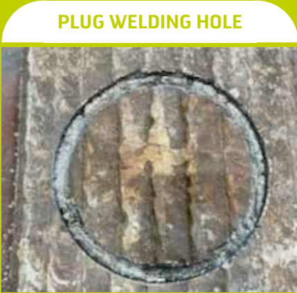
Cut a 125 mm (5") diameter disc from a 10 mm on 10 mm (3/8" on 3/8") Duroxite® 200 plate and weld only the substrate of the disc and hole to the plate using 560 MPa (80 ksi) low alloy joining wire.
