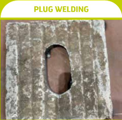
Before welding a Duroxite® 200 10 mm on 10 mm (3/8" on 3/8") plate with an oval hole.
