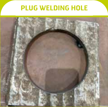
Before welding a Duroxite® 200 10 mm on 10 mm (3/8" on 3/8") plate with a 150 mm (6") diameter hole.
