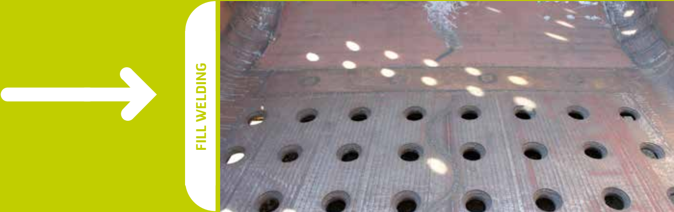
Duroxite® plates welded together with the gaps properly filled between liners to prevent spalling.
