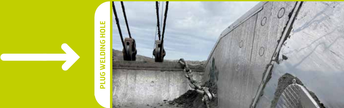
Plug filling of round holes to attach a Duroxite® liner plate on the bucket's inside.
