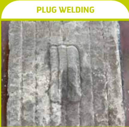
Use 1.6 mm (1/16") Duroxite® 200 Wire to cap the weld with two passes.
