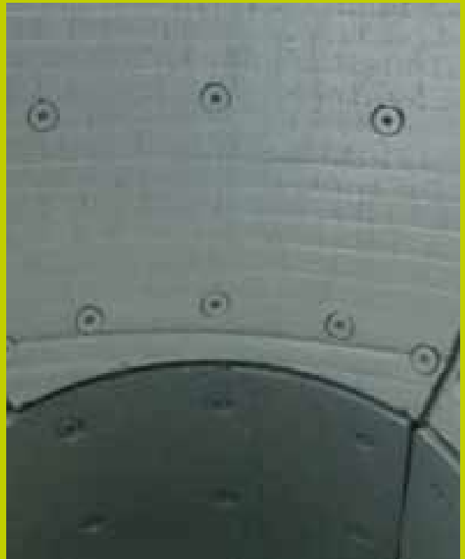
BOLTED LINER WITH MILD STEEL INSERTS
