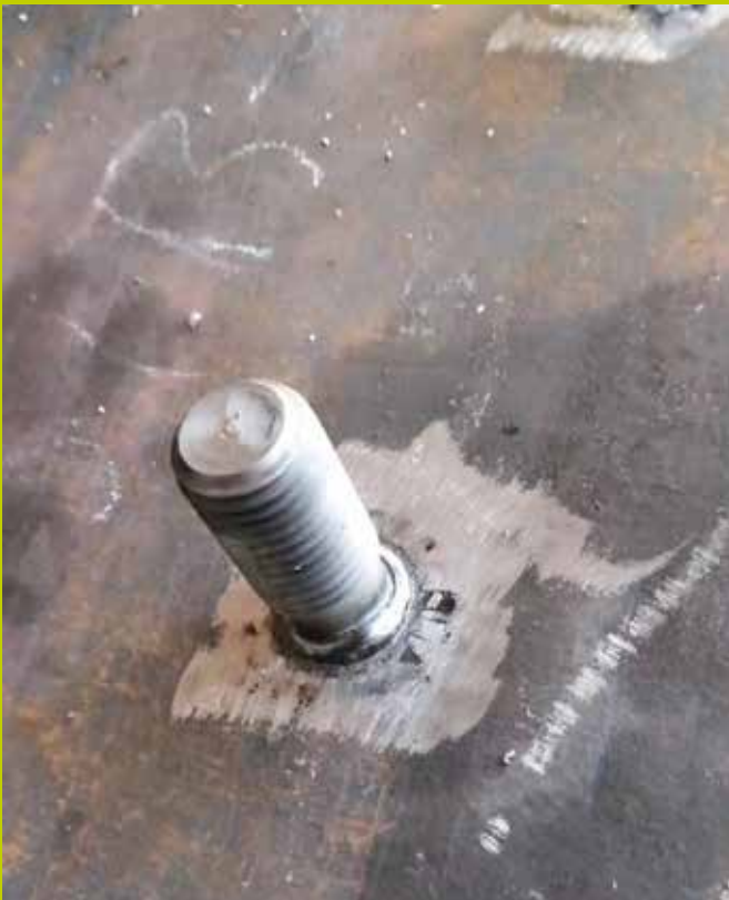
WELDED STUD USED FOR FINAL ASSEMBLY
