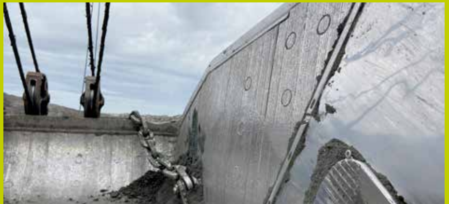
Plug filling of round holes to attach a Duroxite® liner plate on the bucket's inside.
